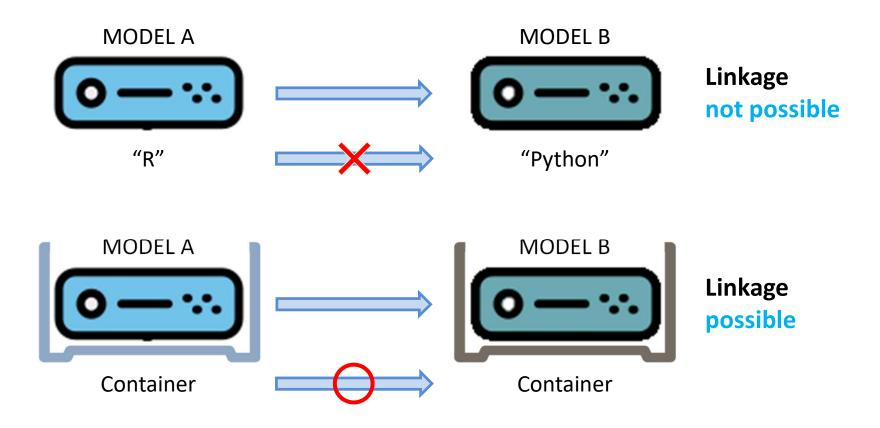
Containers are connected through API.(API: Application Programming Interface)
